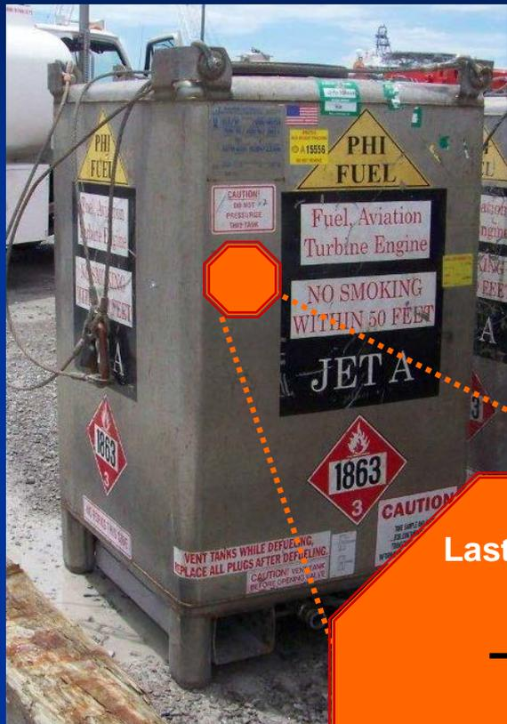
*A decal would be adhered to two sides of the fuel transporter. Forklift side is preferable to improve awareness of loading coordinators and forklift operators, as well as offshore personnel.*
