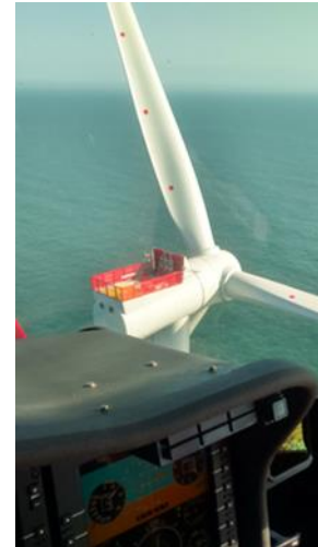
Figure 8-3: Retreating blade horizontal position (alternative SAR position) (Courtesy: UK MCA)
