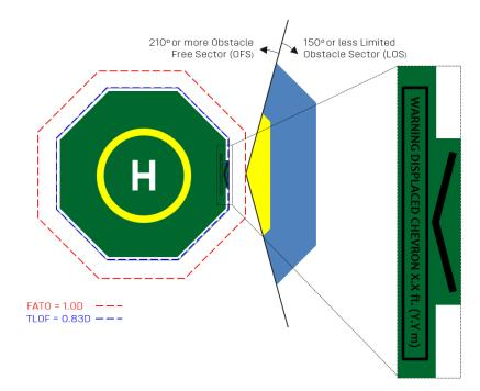
Figure 24: Displaced Chevron Marking
