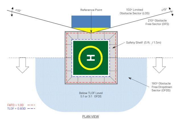
Figure 7: Obstacle Free Sector, Limited Obstacle Sector and Obstacle Free Dropdown Sector for Helideck with 0.83D TLOF
