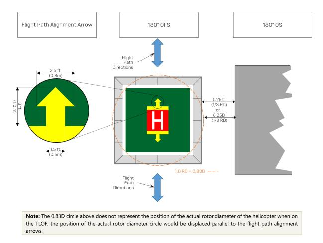
Figure 15: Example of the TDPM for a Square Helideck with a 180° OS
