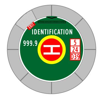
Figure 22: D-value, TLOF Size and Weight Markings for a 0.62D TLOF with a Circular TLOF (i.e., single engine helicopter, like a Bell 206B)
