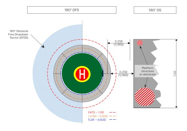
**Note:** The 0.83D circle above does not represent the position of the actual rotor diameter of the helicopter when on the TLOF, the position of the actual rotor diameter circle would be displaced parallel to the flight path alignment arrows.
