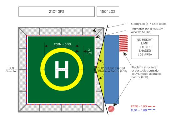
Figure 1: Square Helideck with a 1.0D FATO, a 1.0D TLOF and a 210° OFS/150° LOS
