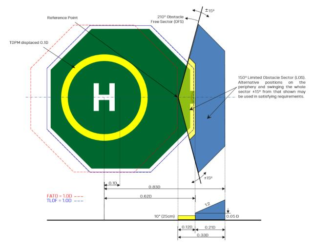
Figure 13: Displaced TDPM for a 1.0D TLOF
