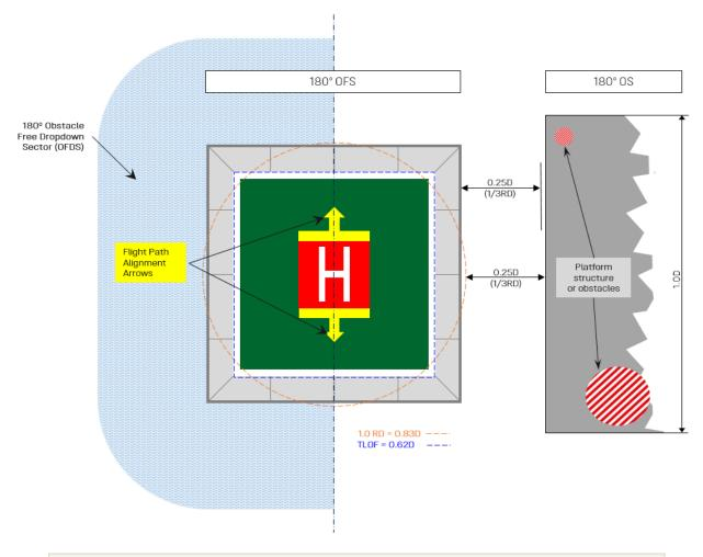
**Note:** The 0.83D circle above does not represent the position of the actual rotor diameter of the helicopter when on the TLOF, the position of the actual rotor diameter circle would be displaced parallel to the flight path alignment arrows.
