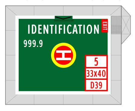
Figure 21: D-value, TLOF Size and Weight Markings for a 0.62D a Rectangular TLOF (i.e., single engine helicopter, like a Bell 206B)
