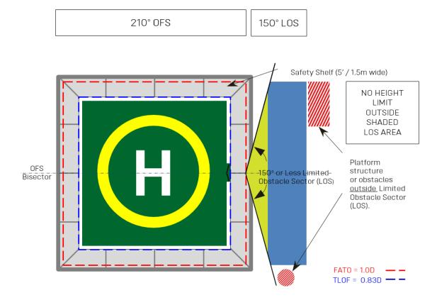
Figure 2: Square Helideck with 1.0D FATO, a 0.83D TLOF and an OFS of 210°
