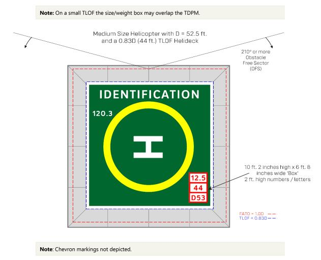
Figure 6-7: Size and weight markings for a 0.83D square helideck
