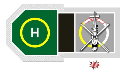
Figure 12-9: 'No Nose' marking and PCOM on TDPC with parked helicopter
