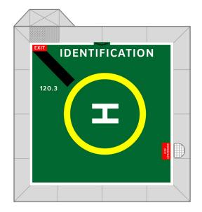
Figure 6-19: Unmanned facility Exit marking with Walkway marking
