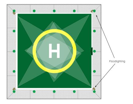
Figure 7-3: Typical Floodlighting arrangement
