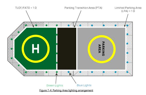
The blue lights on the inboard section of the parking transition area and parking area shall be flush mounted as shown in Figure 7-4.
