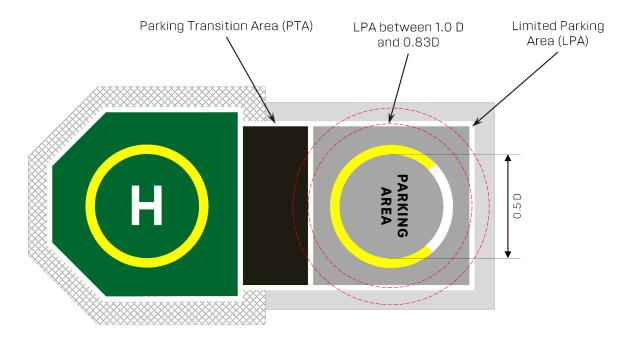
Figure 12-3: Limited Parking Area (LPA) of 0.83D with Parking Circle Orientation Marking (PCOM)
