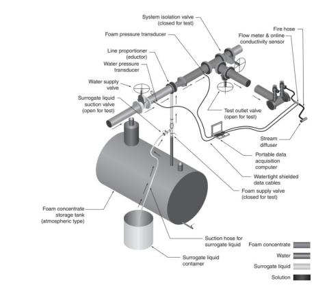
Figure 13-2: Example Configuration for Surrogate Liquid Test Method: Atmospheric Tank and Line Proportioner System<sup>3</sup>
