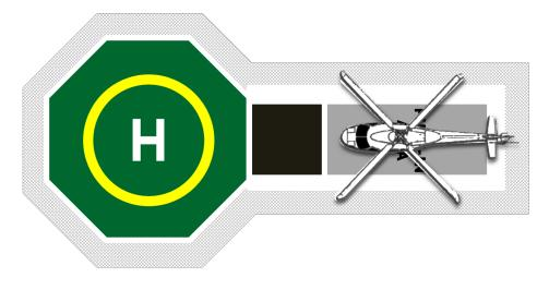
Figure 12-12: Push-In Parking Area (PIPA) with parked helicopter
