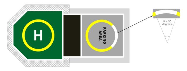
Figure 12-2: Touchdown Parking Circle (TDPC) marking and Parking Circle Orientation Marking (PCOM)
