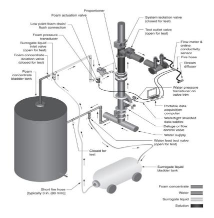
Figure 13-1: Example Configuration for Surrogate Liquid Test Method: Bladder Tank System<sup>2</sup>
