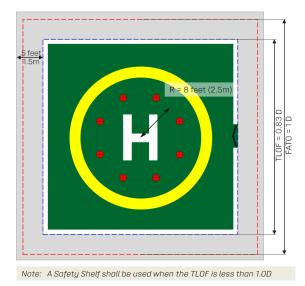
Figure 14-3: Tie-down point arrangement for an offshorebased helicopter on 0.83D TLOF helideck (c)
