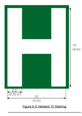
The "H" shall be marked co-located with the TDPM with the crossbar of the "H" lying along the bisector of the obstacle-free sector as shown in Figure 4-2 through Figure 4-5.
