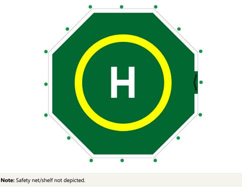
Figure 7-2: Octagon shaped TLOF helideck Perimeter Lighting arrangement
