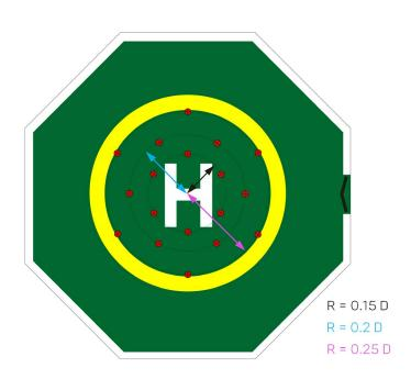
Figure 5-1: Tie down point arrangement
