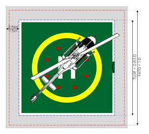
Figure 14-4: Tie-down point arrangement for an offshorebased helicopter on 0.83D TLOF helideck (d)
