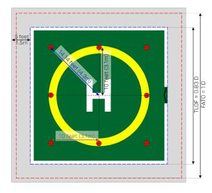
Figure 14-1: Tie-down point arrangement for an offshorebased helicopter on 0.83D TLOF helideck (a)
