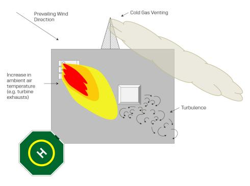
Figure 4-1: Helideck orientation based on wind direction, turbulence, and significant discharge sources
