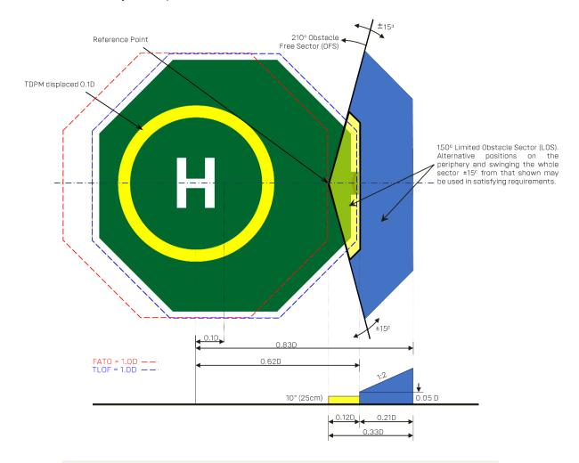
**Note:** Although the first section of the LOS allows for obstacles not exceeding 10" (25cm), there will be a portion of that LOS section that overlaps the TLOF. If objects are required in that overlapping portion over the TLOF, the height above the TLOF surface of those obstacles should be limited to 2 in. (5 cm) (see 4.3.5.2).
