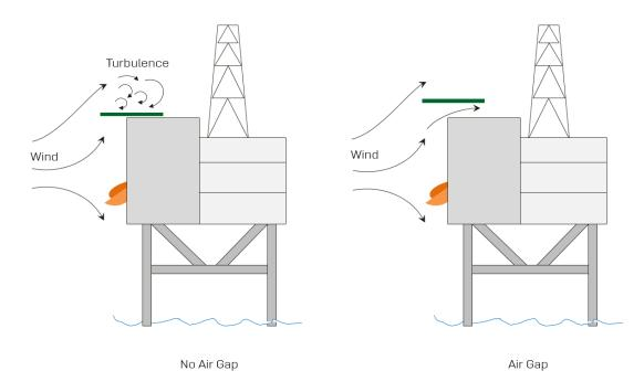
Figure 4-14: Turbulence with and without a helideck air gap
