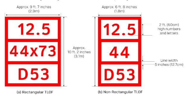
**Note:** Dimensions illustrated refer to 0.83D TLOF designed for a design helicopter with a D-Value of 53 feet and MTOM of 12,500 lbs .
