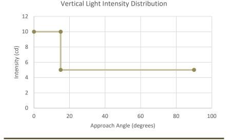
Figure 16-1: Vertical light intensity distribution
