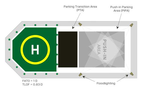
Figure 12-16: Push-in Parking Area (PIPA) lighting arrangement
