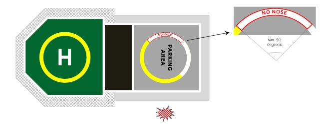
Figure 12-5: 'No Nose' marking and Parking Circle Orientation Marking (PCOM) on TDPC
