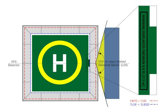
Figure 6-10: Example of a 0.1D displaced TDPM and 'H' for a helideck with 0.83D TLOF and 1.0D FATO
