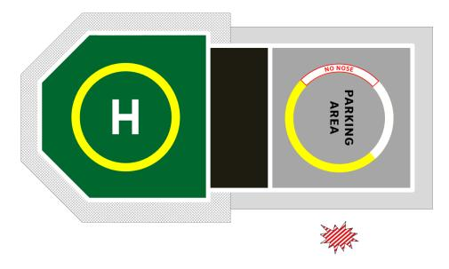
Figure 12-8: 'No Nose' marking and PCOM on TDPC
