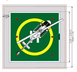
Figure 14-2: Tie-down point arrangement for an offshorebased helicopter on 0.83D TLOF helideck (b)
