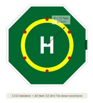
Figure 14-5: Tie-down point arrangement for 1.0D TLOF helideck with less than 40 ft. diameter
