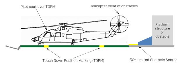
Figure 6-1: Relationship of the TDPM to LOS for a 1.0D TLOF
