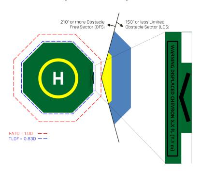
Figure 6-14: Displaced chevron marking
