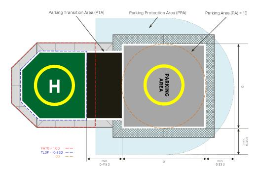
Figure 4-5: 1.0D FATO and 0.83D TLOF with a 1.0D Parking Area
