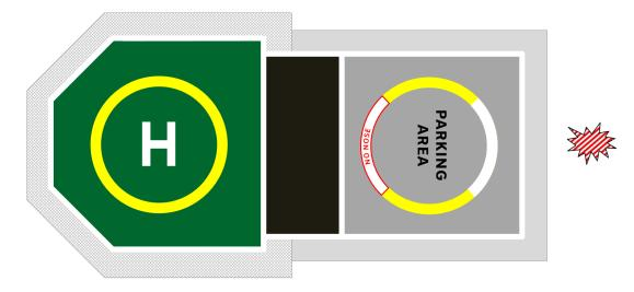
Figure 12-6: 'No Nose' marking and PCOM on TDPC
