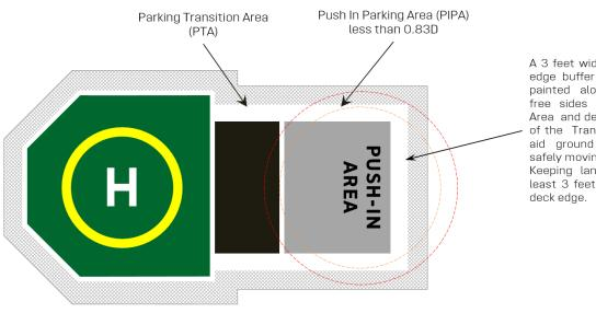
A 3 feet wide, solid white edge buffer line shall be painted along all three free sides of a Push-In Area and deck edge sides of the Transition Area to aid ground handlers in safely moving the aircraft. Keeping landing gear at least 3 feet inside of the deak edge
