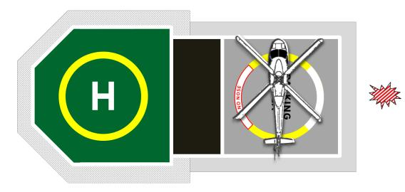
Figure 12-7: 'No Nose' marking and PCOM on TDPC with parked helicopter
