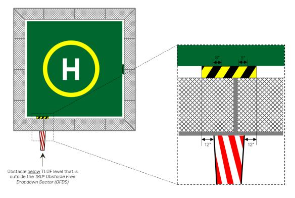
Figure 6-16: Obstacle Warning Marking for OFDS
