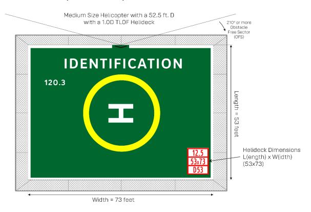
Figure 6-5: Size and weight markings for 1.0D 52.5 ft. medium helicopter rectangular helideck
