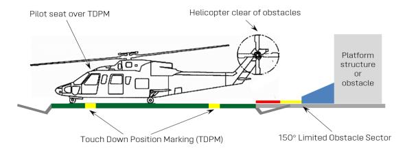
Figure 6-2: Relationship of the TDPM to LOS for a 0.83D TLOF
